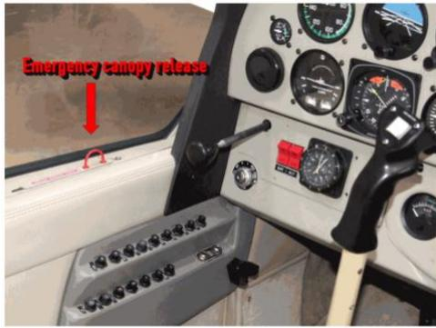
**Emergency release** - There are two emergency release levers at the forward ends of the canopy to allow the canopy to be jettisoned altogether in an emergency. They must never be moved except in an emergency and even then, not in flight!
