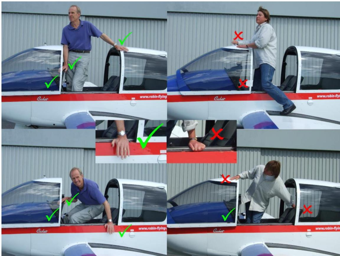
**NOTE: Always open the canopy all the way to its forward stops before getting in or out** - slide it gently, carefully and squarely and do not apply undue force. If it sticks, slide it back towards where you started then try again. Having the canopy fully open is vital to standing up in the aircraft comfortably.
