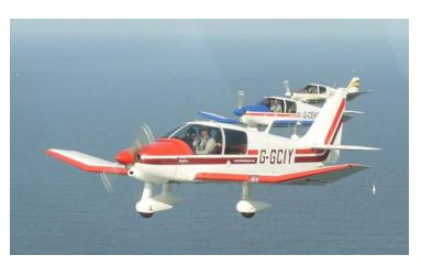
The wide-track undercarriage with highly effective hydro-pneumatic shock absorbers (instead of undamped bendy bits of metal or composite!) flatters the pilot and offers a generous 22 knot published crosswind capability. It also copes comfortably with rough strips allowing full advantage to be taken of the DR400's excellent short field capability.
